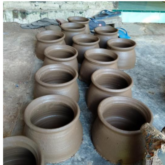
Figure 3. Kendil is a pottery serving as a water or cooking broth container. The wide top makes it easy to take water or broth/soup. The basic shape of the pottery is produced using a simple technique, namely the pinch technique (compression technique). It is made using a plendes or prebot foundation, a ply of wood cut horizontally in the shape of a circle (log cut), and given an axle in the middle so that it can be rotated on its axis (Source: Personal Documentation, 2021.)
