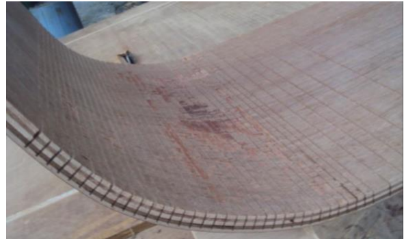
Figure 3. The process of making a drum body from plywood
