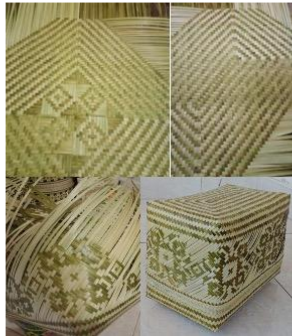
Figure 7. The weaving stage of the bakalan (bottom part) is square (top left), rectangular bakalan (top right), and the muquin for the cemplong motif (bottom left), and the finished packaging design (bottom right). (Source: Des's Document, 2022)
