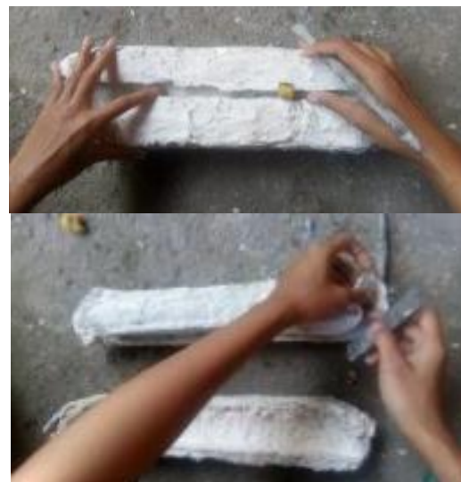
Figure 5. Making mold using silicon
