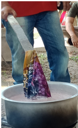
Figure 4. The process of removing wax in boiling water
